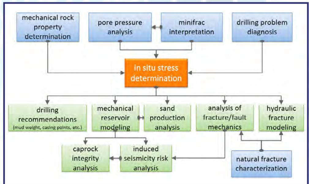
Figure 1. Generalized Geomechanics Workflow and Applications
