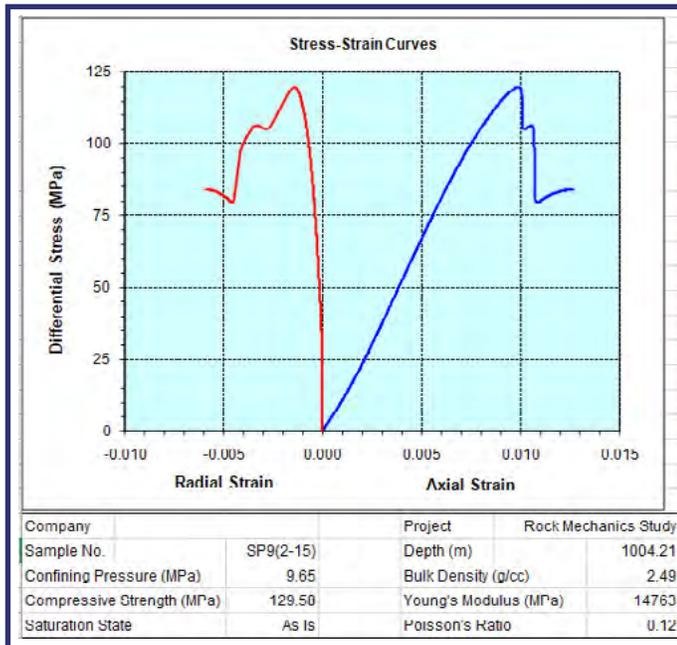
Figure 2. Example of a Rock Mechanics Test on Core
